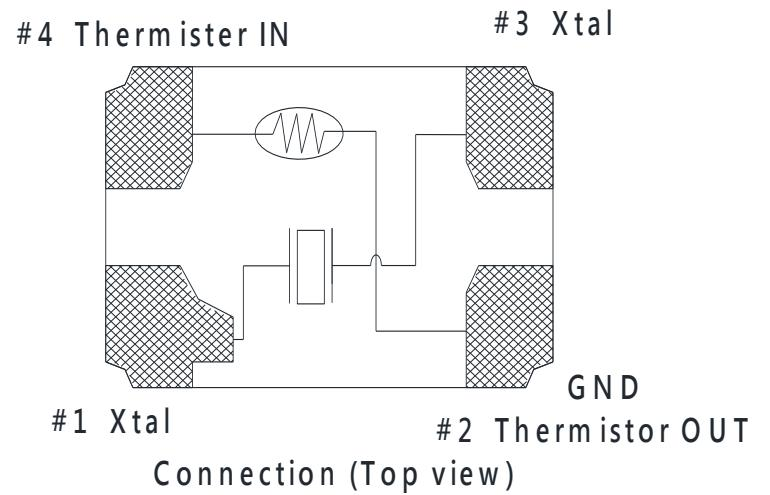
Note: RT2 shall be connected to GND is recommended
